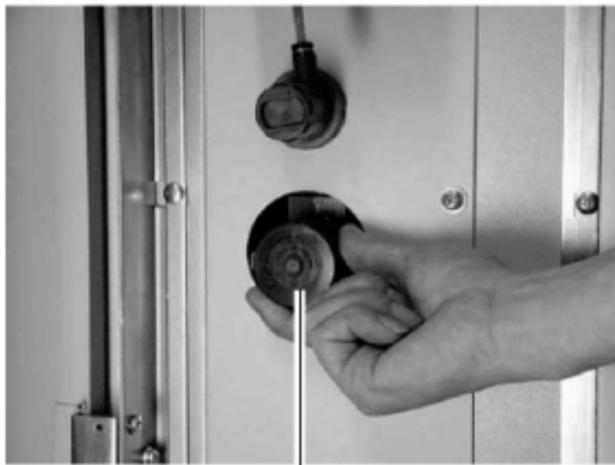
Air supply/shut-off switch
